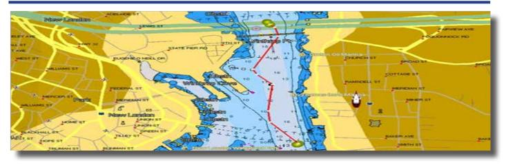
Easy Routing calculates the shortest safe route from start to end points. The proposed route will display a level of safety for each leg, thereby avoiding obstacles such as: Nav-Aids, Rocks, Obstruction, Shallow waters, Dangerous Areas and Bridges. **IMPORTANT:** The suggested route must be checked, edited and approved before using for navigational purposes.
