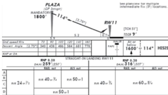
Descent angles are provided so that you do not have to perform additional calculations during critical phases of flight.
